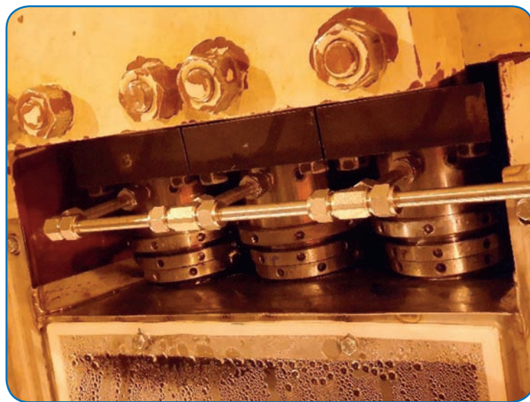
After: the configuration of the drainage tubes has been changed; now they do not impede the tightening of the seals
