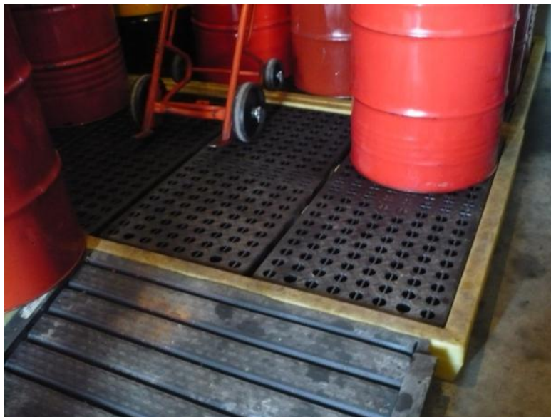
Photo 21 Use of large drip trays at the OPF PMD
