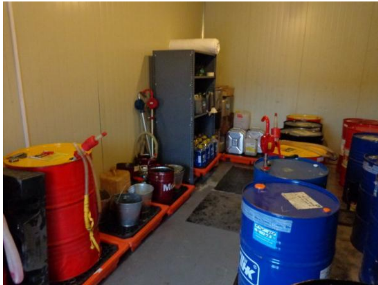
Photo 20 Small volume containers on plastic gridded drip trays
