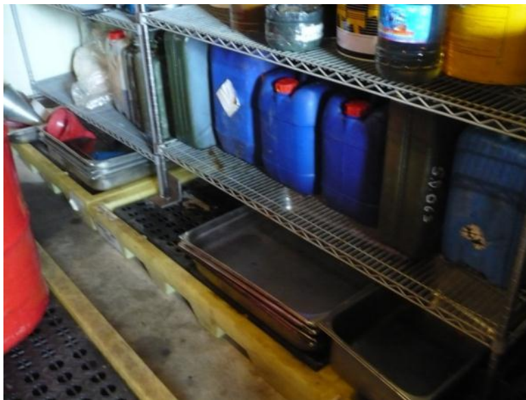
Photo 22 Drip trays under shelving racks
