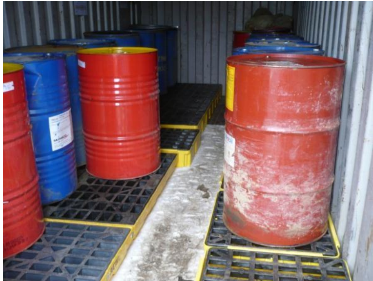
Photo 18 Used oil drums on inadequate secondary containment, Nogliki
