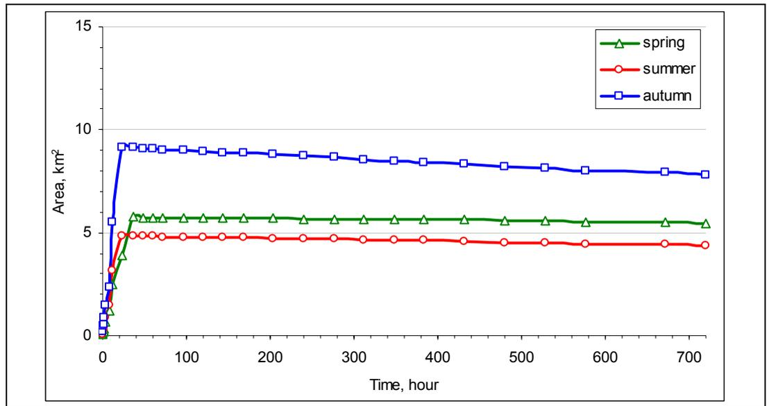
**Figure 2.2** *Excursion Envelopes (Risk Zones) for Oil Spills from Piltun-A Platform (Molikpaq): Autumn (Scenario: Volume: 96m<sup>3</sup>; Cause: Pipeline rupture, REA 2004)*
