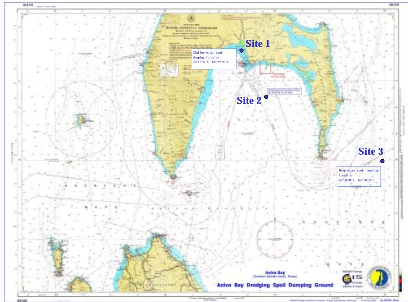
Figure 6.5 Map showing location of proposed sites for the disposal of dredged material arising from LNG associated works in Aniva Bay
