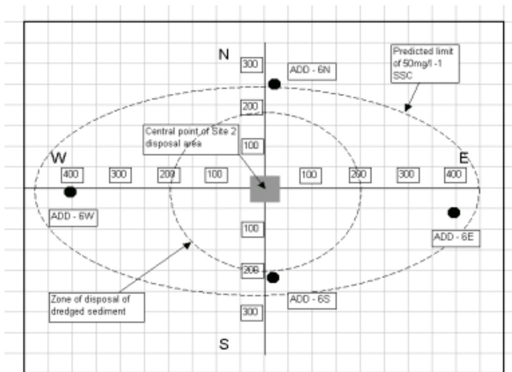
**Figure 6.6** Plot showing Location of Aniva Bay Sampling Stations ADD6 (N,S,E & W) in Relation to Site 2 Disposal Area (data from DVNIGMI 2001). [Note: an approximation of the main area of disposal and modelled limit of 50mg/l suspended sediment concentration (SSC) is shown (derived from the EIA – Vol.5)]
